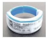
**TLD Ring Dosimeter**: This Ultra Ring<sup>TM</sup> is an extremity dosimeter (ring badge) and is worn on the finger and used to determine shallow-dose equivalent from external sources of gamma, x-ray, and beta radiation to the fingers and hands. The 0.25 MeV cutoff for radiation applies here also. The minimum reportable dose is 20 mrem. Identification is permanently engraved by laser and cannot peel, smear,
